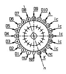
Ref.: 08800009 sp: short pin nc: not connected ic: internal connection
